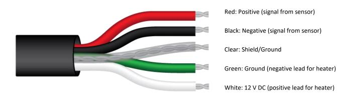
Wiring for SP-510 with Serial Numbers range 1270 and above, and SP-610 with Serial Numbers 1094 and above (or that have cable connectors)
