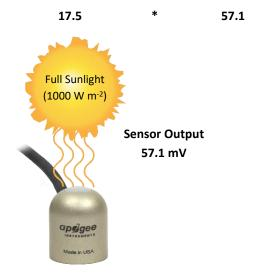
Example of total shortwave radiation measurement with an Apogee SP-510 pyranometer. Full sunlight yields total shortwave radiation on a horizontal plane at the Earth's surface of approximately 1000 W m<sup>-2</sup>. This yields an output signal of 57.1 mV (varies from sensor to sensor). The signal is converted to shortwave radiation by multiplying by the calibration factor of 17.5 W m<sup>-2</sup> per mV (approximately, varies from sensor to sensor).
